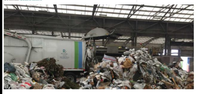
Garbage from homes and businesses stops over at the Metro Central Transfer Station where it's compacted and transferred into long-haul trucks for transport to a landfill 150 miles away.
